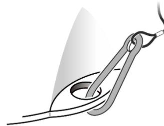
**Figure 6. Safety cable attachment**
