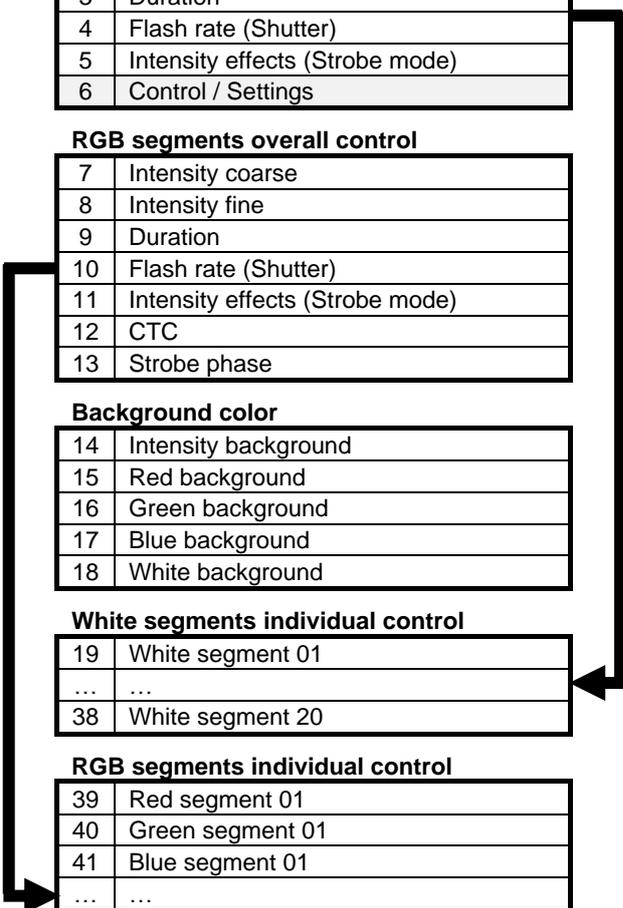
The upper and lower halves of each RGB segment are controlled together, giving individual RGB control of 20 RGB pixels in total.
