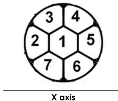
The drawing above shows the standard pixel layout with the fixture standing on the ground, pan at 50% (home position) and tilt at 50% (front).
