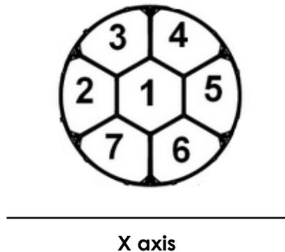
The drawing above shows the standard pixel layout with the fixture standing on the ground, pan at 50% (home position) and tilt at 50% (front).
