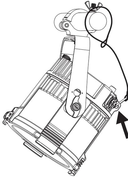
**Figure 3. Safety cable attachment point**
