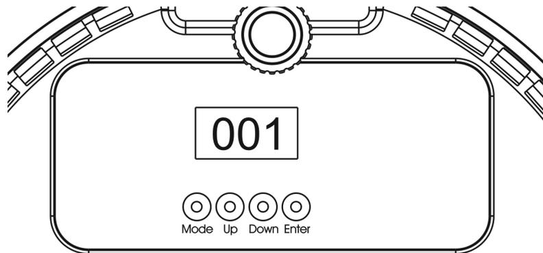
**Figure 9. Onboard control panel**
